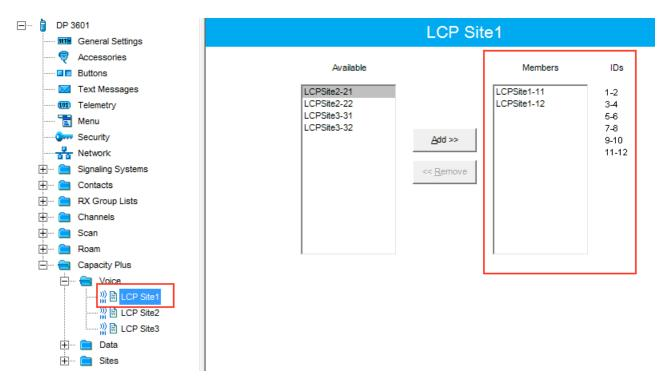
Please note that **ID**s in the **Members** list should correspond to **Slot 1 ID Channel** and **Slot 2 ID Channel** specified in repeater settings.
