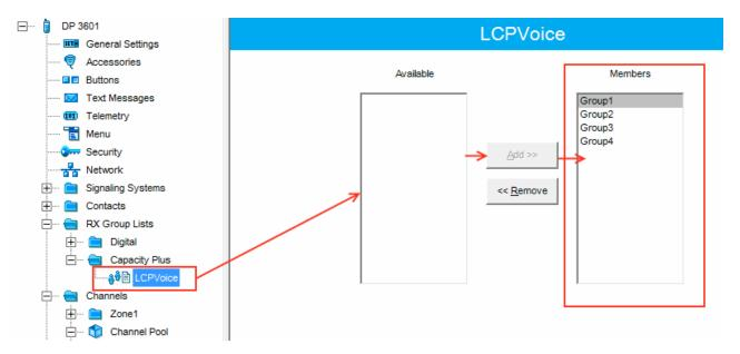
5. Add all repeaters, which are in the LCP system, to the **Channel Pool**. The color code should equal the color code specified for repeaters. In our case **Color Code**=1.
