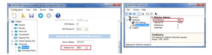
The PORT SU field (Interfaces > ARS Settings) in MOTOTRBO DDMS Administrative Client matches the ARS UDP Port field in MOTOTRBO Network Interface Service Configuration Utility (Advanced > Networks).
