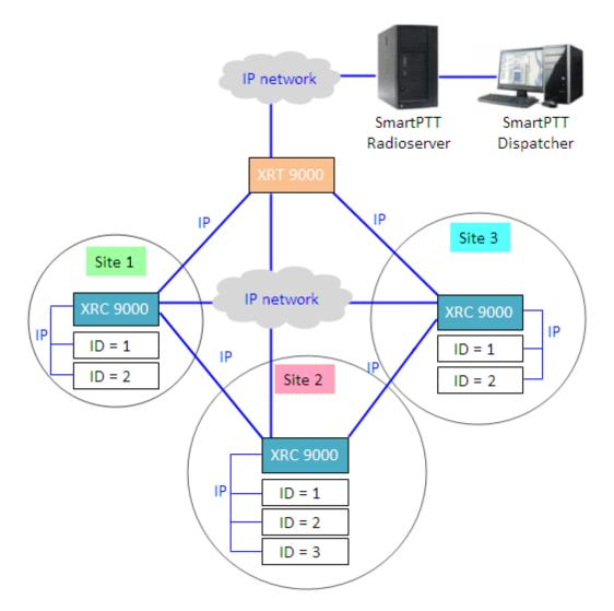
In this network there is only one XRT 9000 Gateway in the network system, and one XRC 9000 Controller per site. The number of repeaters per site can be different. In this case there are two and three repeaters on site. XRT 9000 joins the MOTOTRBO Connect Plus system as another multi-site XRC 9000 Controller peer. XRT 9000 creates a pathway between the radios on a Connect Plus system and the third party application, in our case it is SmartPTT Radioserver.
