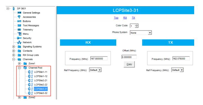
6. Create Voice lists and Data lists according to the amount of sites. As all of our repeaters are Trunk repeaters (transmit voice and data), create only Voice lists. When adding new Voice list, under the Available list you can see all the channels which were added to the Channel Pool. So, for *Site 1* add a Voice list (LCP Site 1) and add *LCP Site 1-11* and *LCP Site 1-12* to this list.
