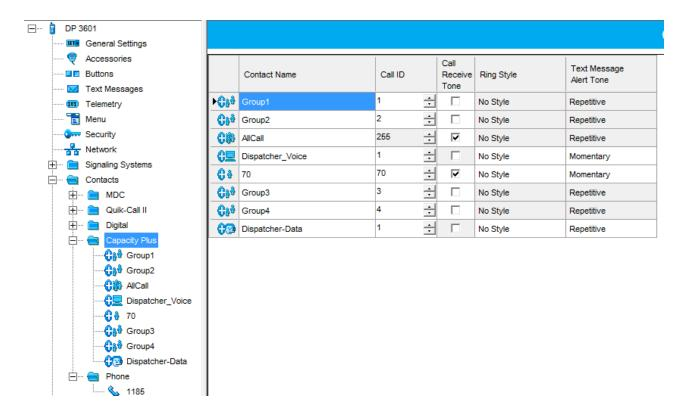
Also, add **Dispatcher Call** for transmitting data to SmartPTT Radioserver and **PC Call** to be able to initiate calls to SmartPTT Dispatcher. Make sure that the **ID**s of these calls equal **Slot ID** in SmartPTT Radioserver Configurator (see <u>SmartPTT Radioserver configuration</u>).
