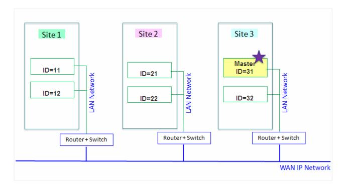
Each radio ID, either subscriber radio ID or repeater ID should be unique in the radio system. In this example you can see 2 repeaters with ID's *11* and *12* on *Site 1*, 2 repeaters with ID's *21* and *22* on *Site 2*, and 2 repeaters with ID's *31* and *32* on *Site 3*. The repeater with ID=*31* is a Master.
