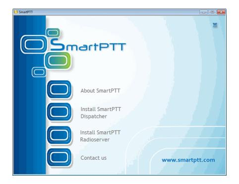
3. Install SmartPTT Radioserver first and then SmartPTT Dispatcher. For both installation processes the setup wizard will be used.
