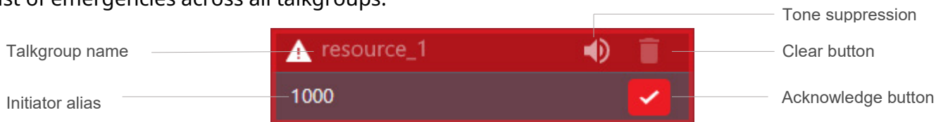
Figure 29: Console-wide Emergency Panel
