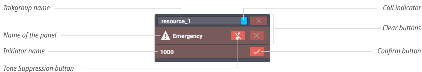
Figure 27: Console-wide Emergency Panel
