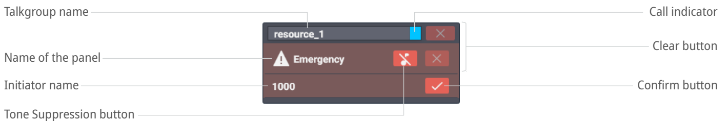
Figure 56: Console-Wide Emergency Panel
