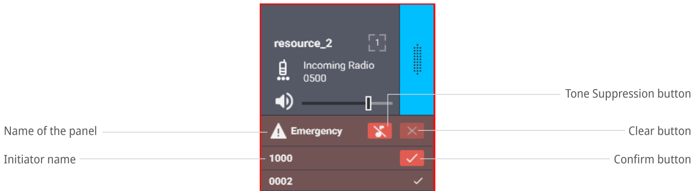
Figure 45: Emergency Panel on Talkgroup Tile
